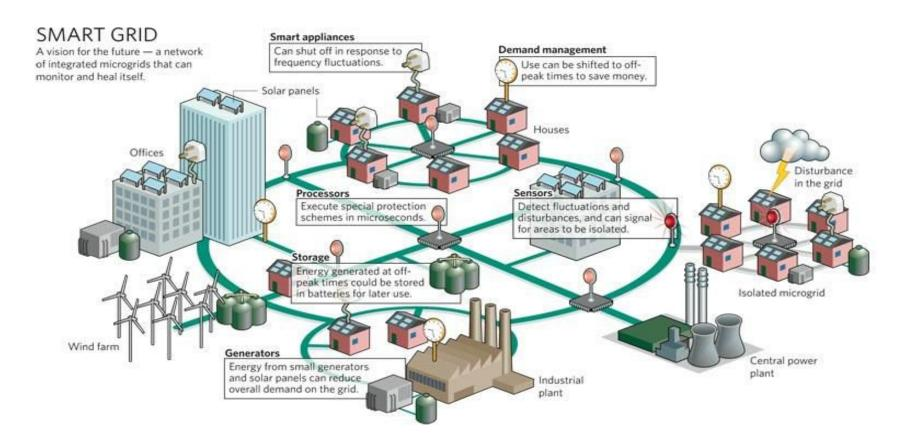
One view of smart grid is as a linking of multiple semi-autonomous micro grids
