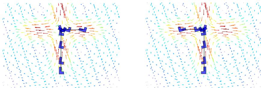
FIG. 5.2. *Enantiomer separation of a right-handed (left) and left-handed (right) L-shaped enantiomer at the central streamlines. The right-handed L-shaped particle follows the vortex rotating counter-clockwise in the upper right quadrant whereas the left-handed L-shaped particle follows the vortex rotating clockwise in the upper left quadrant.*
