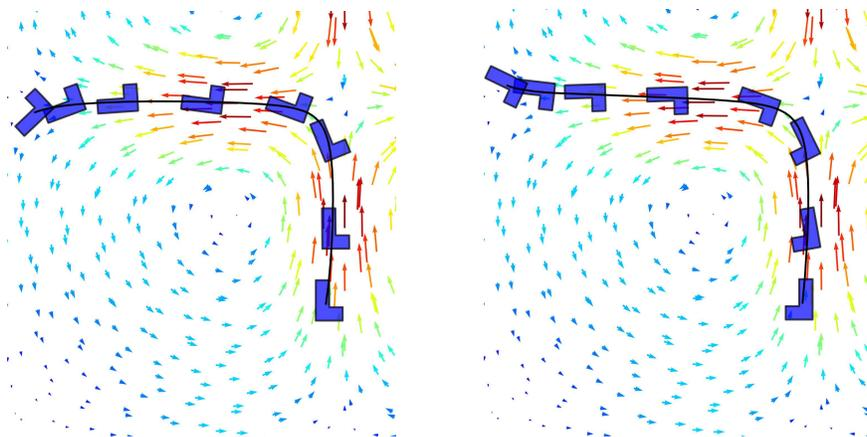
FIG. 5.1. *Enantiomer separation of a right-handed (left) and left-handed (right) L-shaped enantiomer at the outgoing velocity streamlines. The right-handed L-shaped particle follows the vortex rotating counter-clockwise in the lower left quadrant whereas the left-handed L-shaped particle follows the vortex rotating clockwise in the upper left quadrant.*
