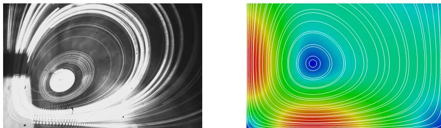
FIG. 4.4. *Left: Experimental SAW generated surface streaming profile with operating frequency  $f_{IDT} = 1.42 \cdot 10^2$  MHz of the IDT. Right: Simulated vorticity pattern generated by a quadrupolar force field with  $v_{max}(f_{IDT}) = 2.0 \cdot 10^{-3}$  m/s.*
