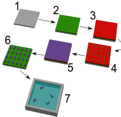
FIG. 4.3. *Schematic representation of fabrication of the photoresist particles. 1) Clean silicon wafer. 2) A sacrificial layer of omnicoat is applied 3) SU8-2 is applied. 4) Photoresist is partially exposed. 5) Unexposed SU8-2 is developed. 6) Surface is treated with silane. 7) Lift-off. Afterwards particles are transferred onto the water surface and float stably in a well defined orientation.*
