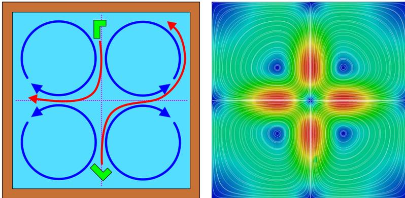
FIG. 1.1. Sketch of the anticipated separation process of L-shaped enantiomers by pairwise counter-rotating vortices (left) and employed vorticity pattern (right).
