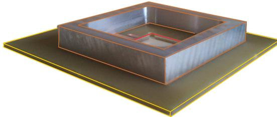
FIG. 4.1. Side-view of the experimental setting (shown without water). The setup is mounted on a circuit board consisting of the fluid container and the IDT with substrate layer in the middle on the bottom of the water bulk.
