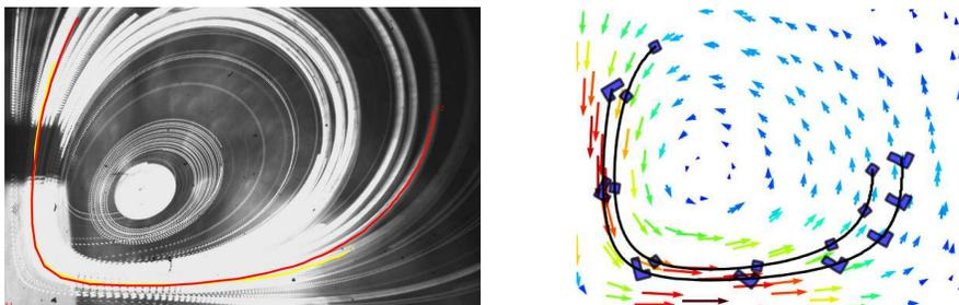
FIG. 4.5. *Left: Experimentally measured trajectories of a square shaped particle (red line) and an L-shaped particle (yellow line). Right: Computed trajectories based on the data of the experimental set up.*
