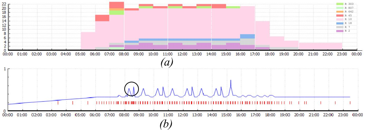
Fig. 6: (a) the bus services provided at a user selected top. Different color blocks show the numbers of buses of the respective routes that provide services at the stop. (b) the service overlap function at a selected stop.
