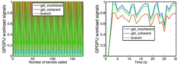
**Figure 2: The original recorded GPGPU workload signals (only showing a 2 seconds portion due to the signal density) and the resampled GPGPU workload signals (30 seconds) when one NVidia CUDA SDK sample (N Body Simulation) ran on the GPUs. For the sake of clear illustration, we only plot three selected GPGPU workload variables: *gld\_incoherent*, *gld\_coherent*, and *branch*.**
