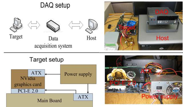
**Figure 1: Data acquisition setup used in this work.** Note that the graphics card had two power supplies (ATX and PCI-E 2.0). DAQ is a FLUKE Hydra logger 2625A power acquisition system, and the target computer is equipped with the chosen NVidia GeForce 8800 GT graphics card (200 Watt power specification), AMD Athlon 64x2 3.0GHz Dual-Core Processor, 2GB memory, and Corsair TX750W power supply.
