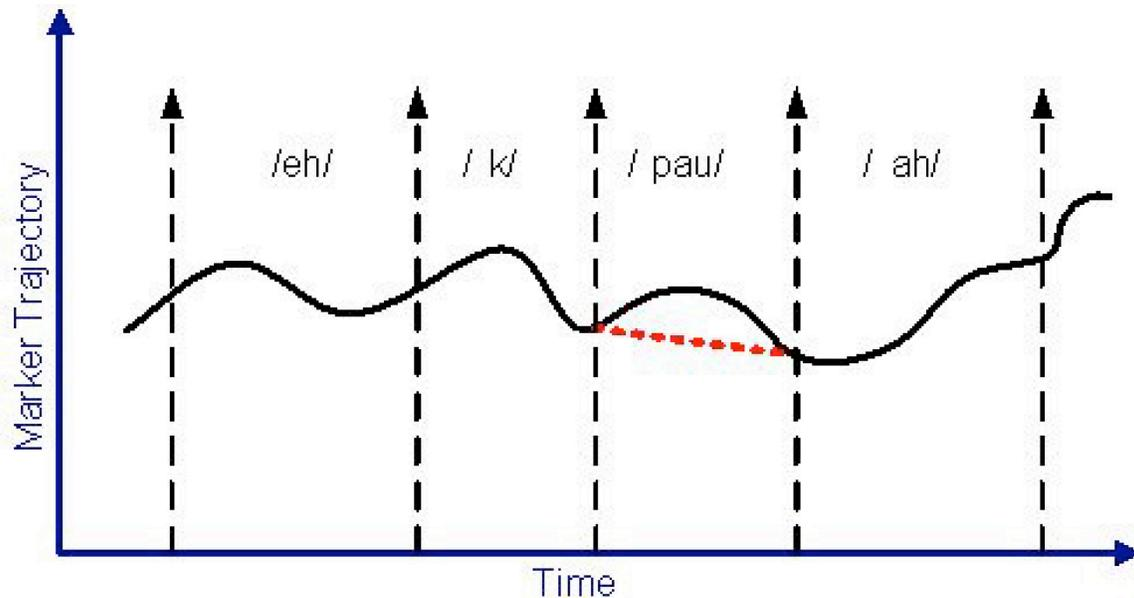
Fig. 13. Illustration of the postprocessing step for the silence time (the /pau/ phoneme time). Here red dot line represents regenerated marker trajectory.
