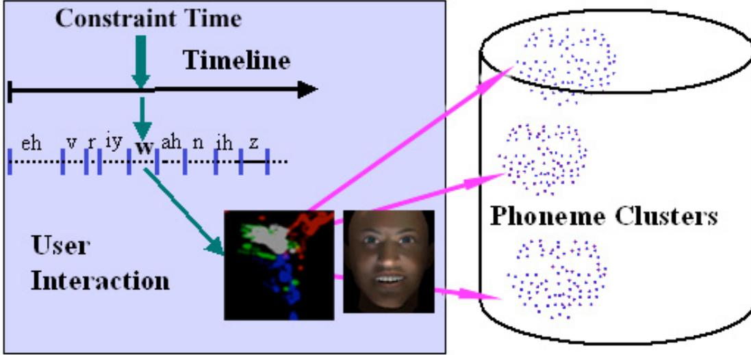
Fig. 8. Illustration of how to specify a motion-node constraint via the phoneme-Isomap interface. When users want to specify a specific motion node for expressing a particular phoneme utterance, its corresponding phoneme-Isomap is automatically loaded. Then, users can interact with the system to specify a motion-node constraint for this constrained phoneme.
