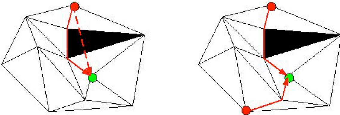
Fig. 12. The left panel compares mesh distance (solid red line) with the direct Euclidean distance (dotted red line) from the source marker/vertex (red spot) to the target vertex (green spot). The black area represents a hole in the face geometry. The right panel shows how the motion of one vertex is calculated based on the propagated motion from several neighboring markers.
