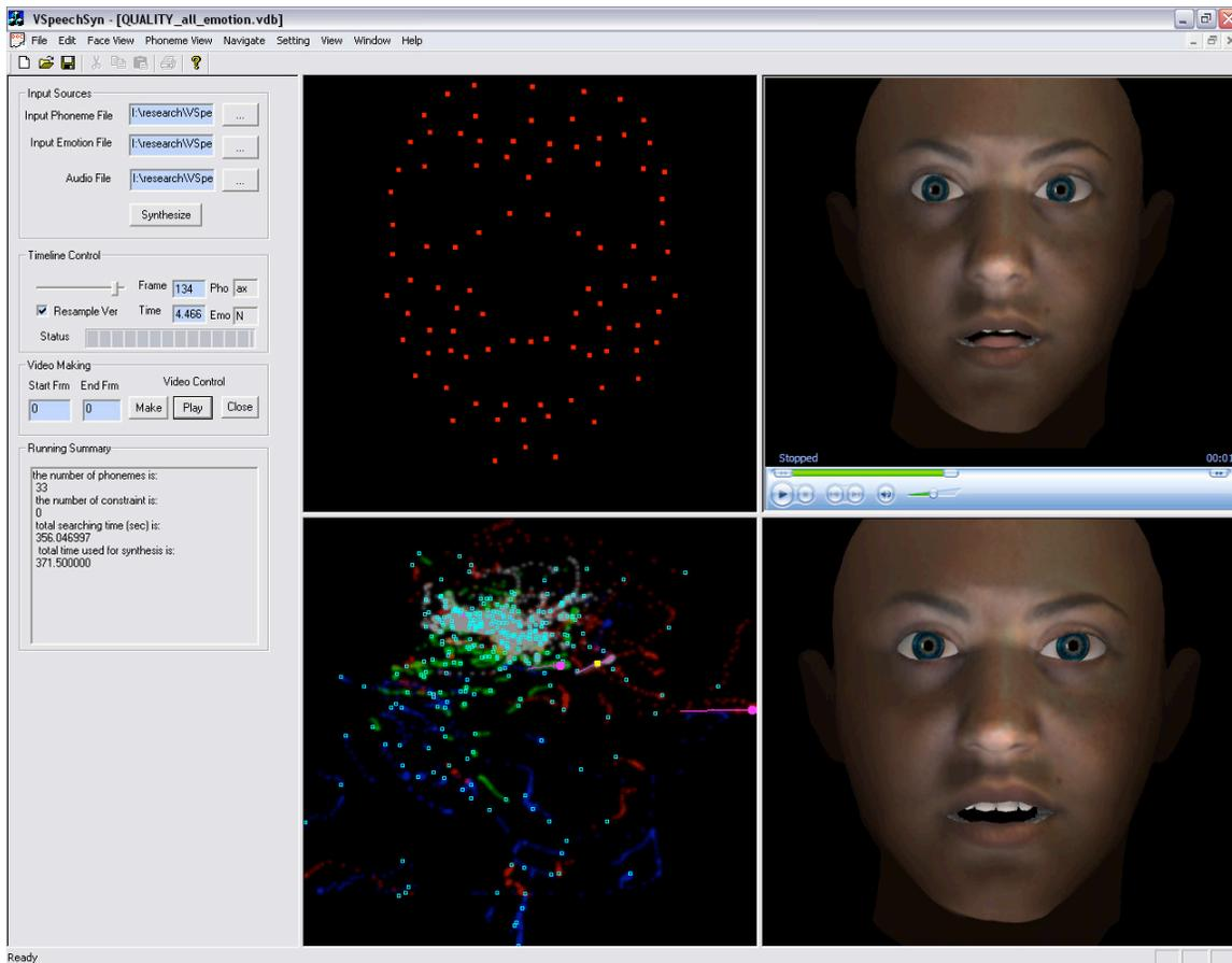
Fig. 14. A snapshot of this running system. The left is a basic control panel, and the right panel encloses four working windows: a synthesized motion window (top-left), a video playback window (top-right), a phoneme-Isomap interaction window (bottom-left), and a face preview window (bottom-right).
