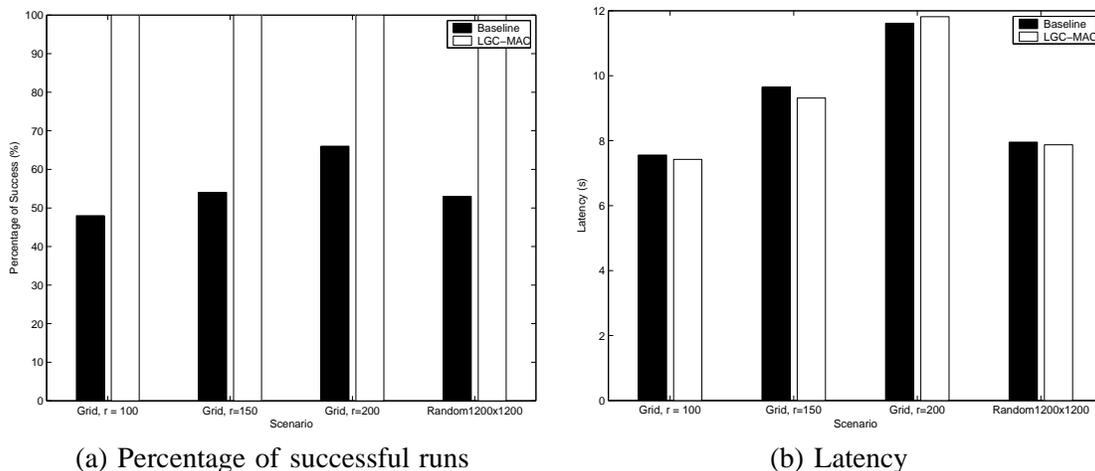
Fig. 10. Propagation of Information with Feedback. Num. of nodes = 100, wireless transmission range = 250
