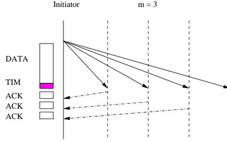
Fig. 2. Illustration of a successful *1-to-m* communication
