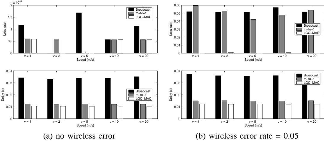
Fig. 8. Acoustic target tracking with and without wireless errors in 60x3 mesh networks
