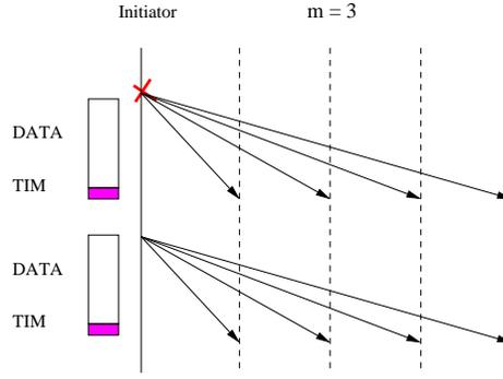
Fig. 4. Illustration of a scenario where the initiator failed to transmit the data message at its network interface. In this case, the initiator needs to retransmit the data frame.
