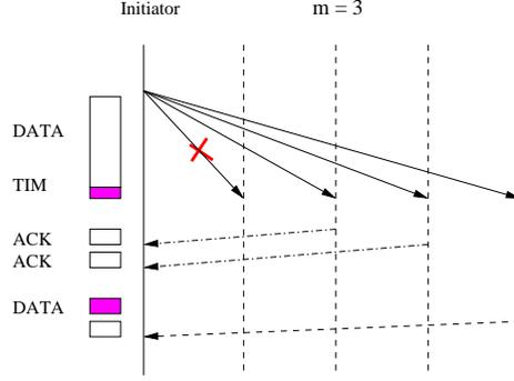
Fig. 3. Illustration of a scenario where some sensors failed to receive the data message. Loss is detected at the initiator. A data frame with no payload is transmitted to solicit further ACKs.
