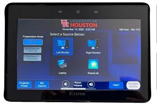
The laptop button is for any device outputting or connecting from HDMI. Devices using USB-C or other outputs will require an adapter.
