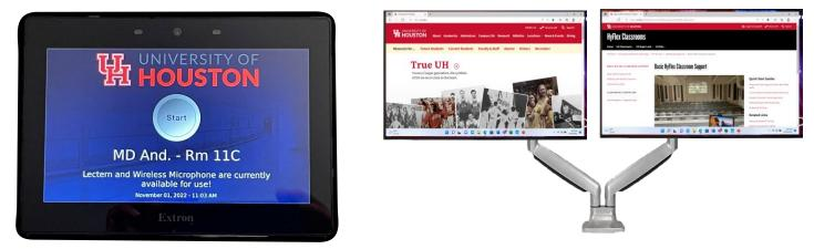
The two monitors will always display the PC when the system is in an OFF state. The left monitor will always show the main PC window and the right monitor can change between Window's sources. The right monitor will not be projected as the main source since it is not the main PC window.
