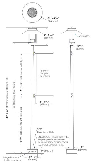
**Note:** Base cover shall rest directly on top of concrete footing and fully cover anchoring hardware. Adjust leveling nuts and trim excess anchor bolt projection as required.
