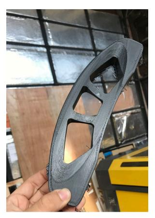
The prototype of the Zero MAS was fabricated using rapid prototyping manufacturing techniques. Using a laser cutter to make the cross member and 3D printing for the other cross member.
