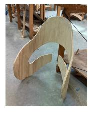
Step 3: Laminate the wood using water-proof, slow drying wood glue, and secure with ratchet straps. Then, demold after 24 hours.
