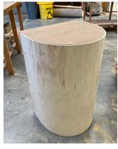
Step 1: Build the mold out of MDF and bendable plywood, then apply saran wrap.
