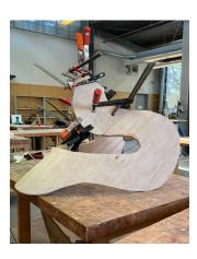
Step 4: Using the same mold, laminate the legs and trim legs to shape. Then, glue to the main body of the chair.
