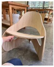
Step 5: Make a mold for the seat and use the same lamination process. Trim and attach the seat using right angle brackets.
