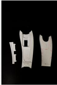
Several full-size prototypes of the thigh part were made. During the iterations, the design of the connection between it and the existing brace was determined, which lead to the completion of the structure of the thigh part.
