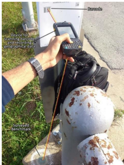
Fig. 4. The device, the benchmark and the barcode.
